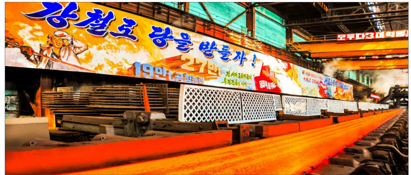
Lumps of structural steel flow through rollers at the Kim Chaek Iron and Steel Complex.
